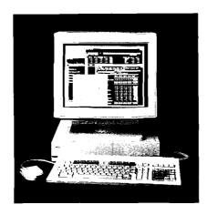
The HP 700/RX Models 17Ci and 17Ca (P/Ns C2706B and C2710B) are new HP X station models that come standard with 17-inch, flickerfree, ergonimically designed, color, Sony Trinitron monitors and 4 MB of user memory.
